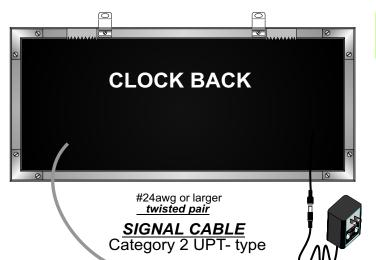
THE PC IS USED TO SET THE LOCATION DISPLAY AND TIME. THE CLOCK CAN RUN ON ITS ON WITHOUT THE PC.
